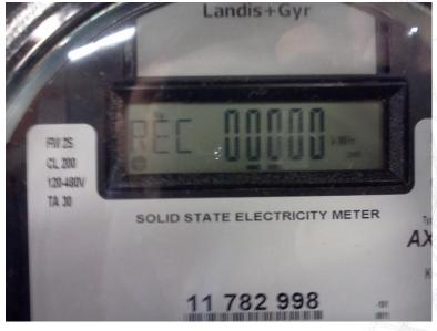
The meter will display "DEL" on the left hand side of the LCD display to indicate the cumulative amount of energy supplied to the member by CPI. The meter will display "REC" on the left hand side of the LCD display to indicate the cumulative amount of excess energy that has been generated by the member and returned to CPI's power grid. This is not the total amount of energy generated by the member but only the remainder of the generated power after the member energy needs have been met.
