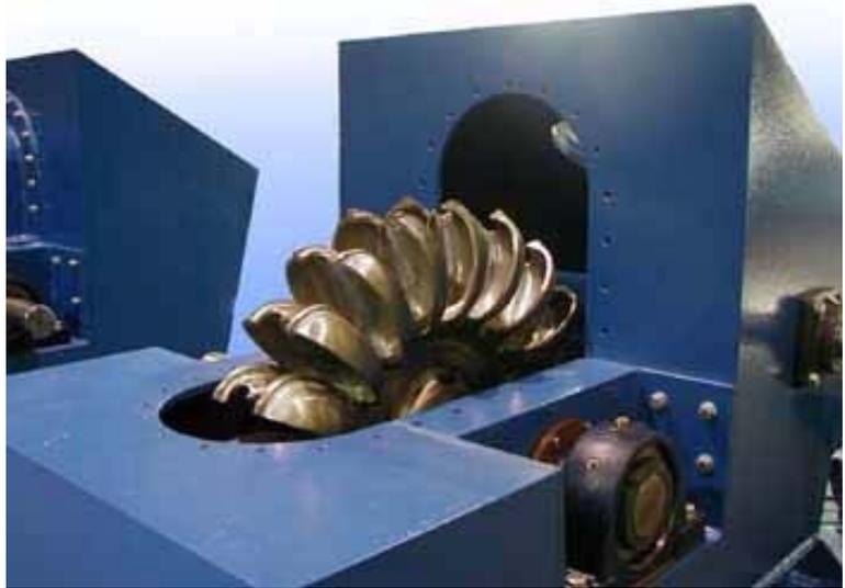
*Pelton-type impulse turbine with housing cover removed.*
