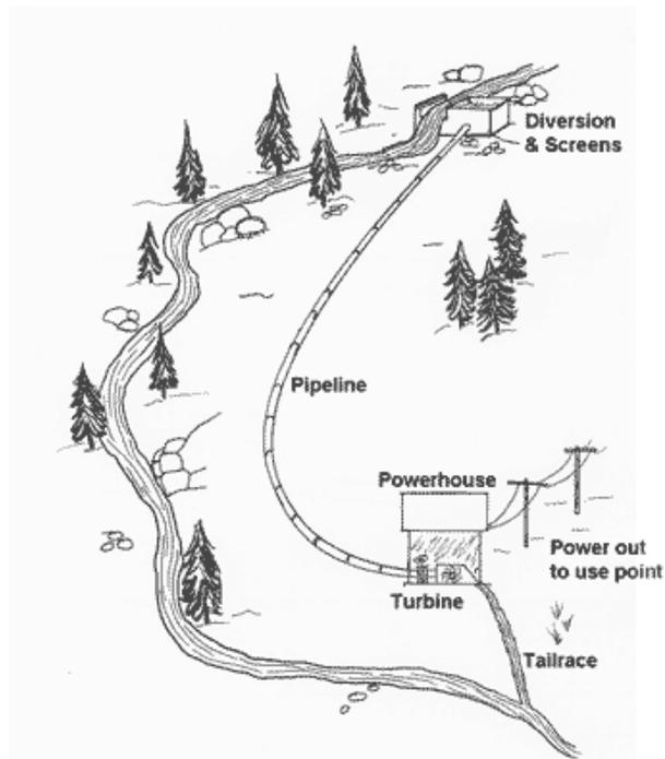
*Major components of a hydro system include a water diversion, pipeline to create pressure, turbine & generator, tailrace for exiting water, and transmission wires.*
